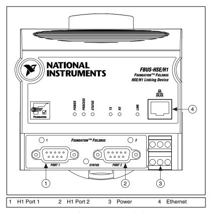
Figure 2-4. Connectors on the FBUS-HSE/H1 LD
